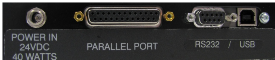
Figure 3: Connectors for power supply, printer (parallel), and computer (serial RS232 or USB), located on the reader's rear panel
