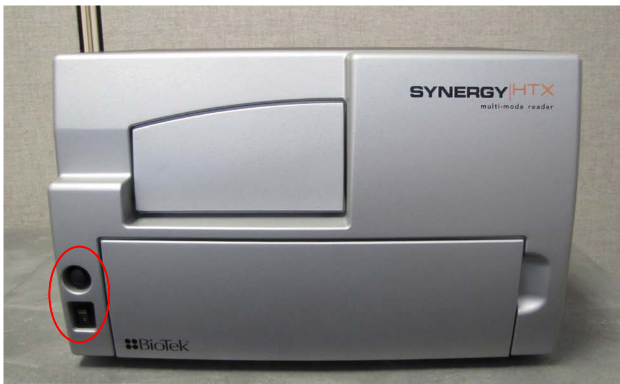
Figure 9: Carrier eject button (top) and power ON/OFF switch
