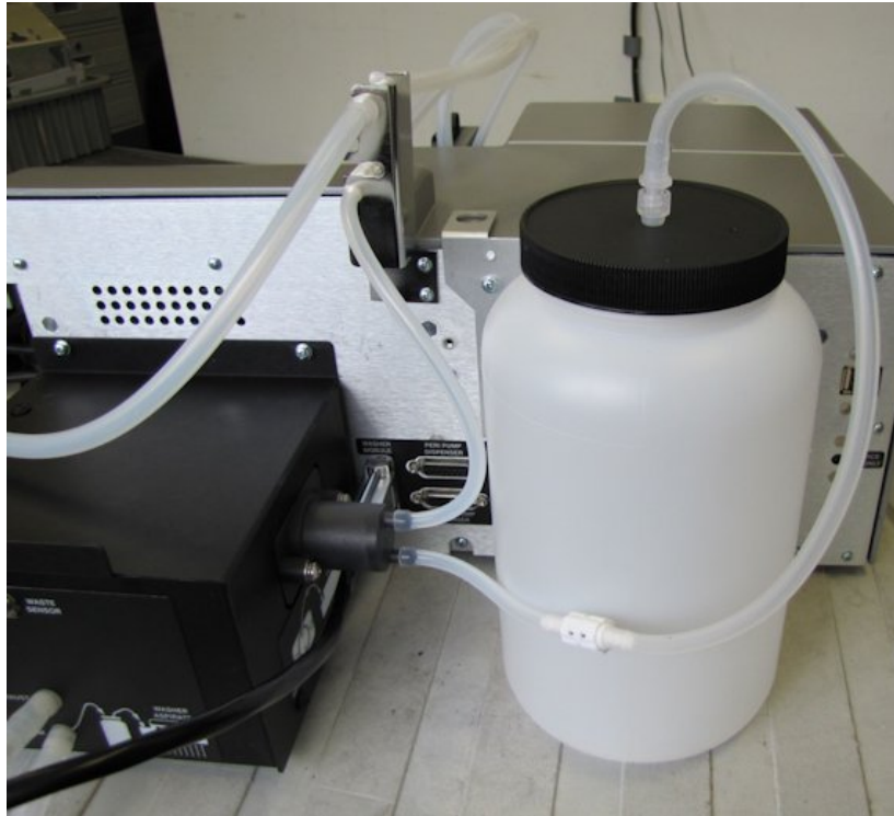
Fluid supply installed
