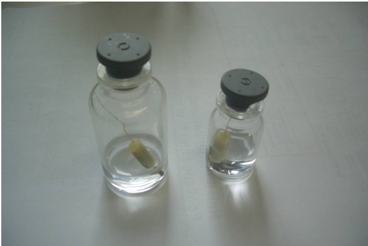
Figure 3-80: Incorrect “immersed” positioning of TEMPRIS sensors in the vial
