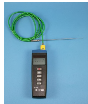
MIN/MAX digital thermometer with add. temperature sensor
